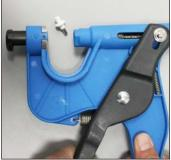
5. Reopen the chamber and remove the punch from the applicator. Check that sampling has been successful (red plunger is visible, sample is in fluid in punch). Remove the used cutter from the applicator by pulling the handles apart. Discard carefully as the cutter is very sharp.
