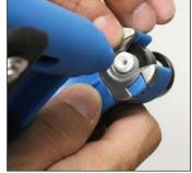
Remove the red plastic clip by pulling it outward. Be careful as the metal cutter above the clip is very sharp. Ensure the applicator is loaded with an unused green punch (if the red plunger is visible, the punch is used and should be replaced with one that is unused).
