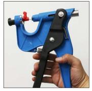
Rotate the black chamber to lock the punch into the device. Carefully squeeze the applicator handles together, guiding the punch tip into place if necessary. When the gun bolt rests flush against the red plastic clip, release the handle.
